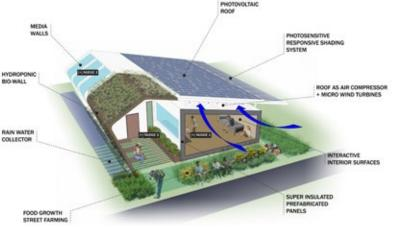
energy collection and dispersal via both sun and wind: a top layer of photovoltaics covers a second layer of mini wind turbines. Neighbor-friendly gardens in the front yard put healthy food front and center, meanwhile, and a hydroponic bio wall serves the dual purpose of shading the front walk and filtering the air. Rain barrels and small pathways channel water and irrigate the gardens.
